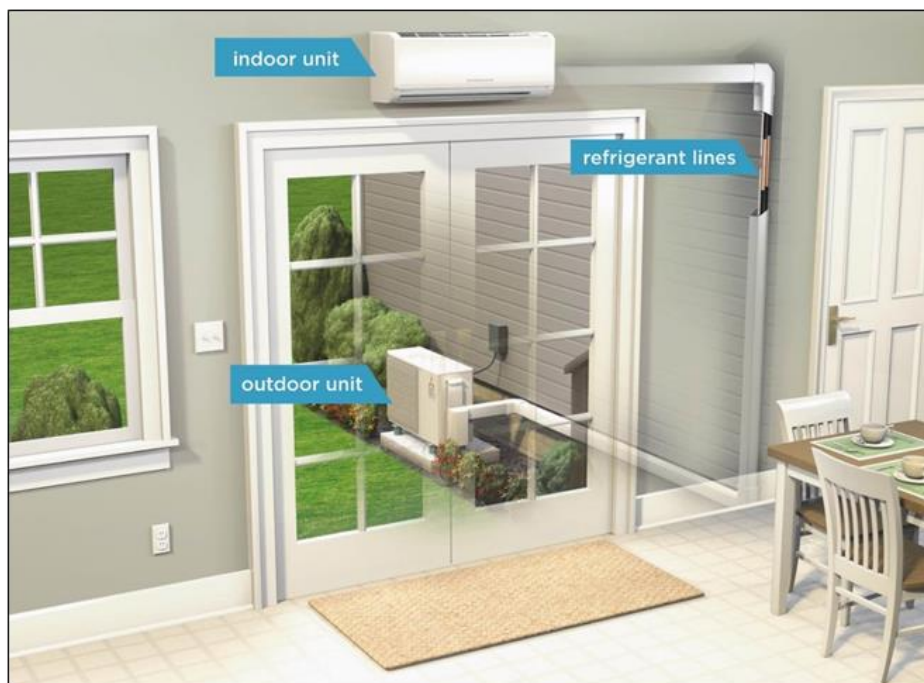
Figure 1. Diagram of an air-source heat pump (mini-split) 13
