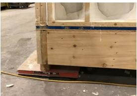
Figure 7. Air pads Utilized to Move Modules Throughout Factory.
